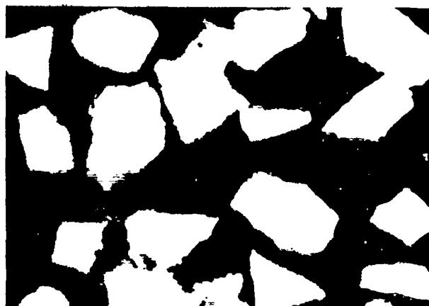
^{238}\text{PuO}_2 - \text{ThO}_2 Particles
